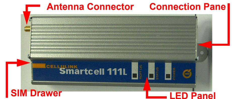
Figure 1: IP Gear Quasar 111L Components
